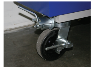
Rear Wheel System with release and brake.
