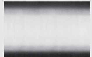
Latex paint through a HEA 517 tip at 1,000 PSI
