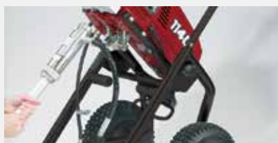
3. Pull handle under body. Slide out fluid section.
